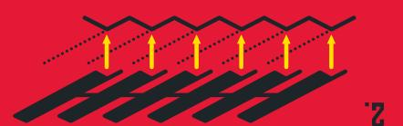
The core element of our patented TRU-Infrared<sup>IM</sup> Technology is the emitter plate. For it to absorb all the heat effectively, it must be positioned flush over the burners.
